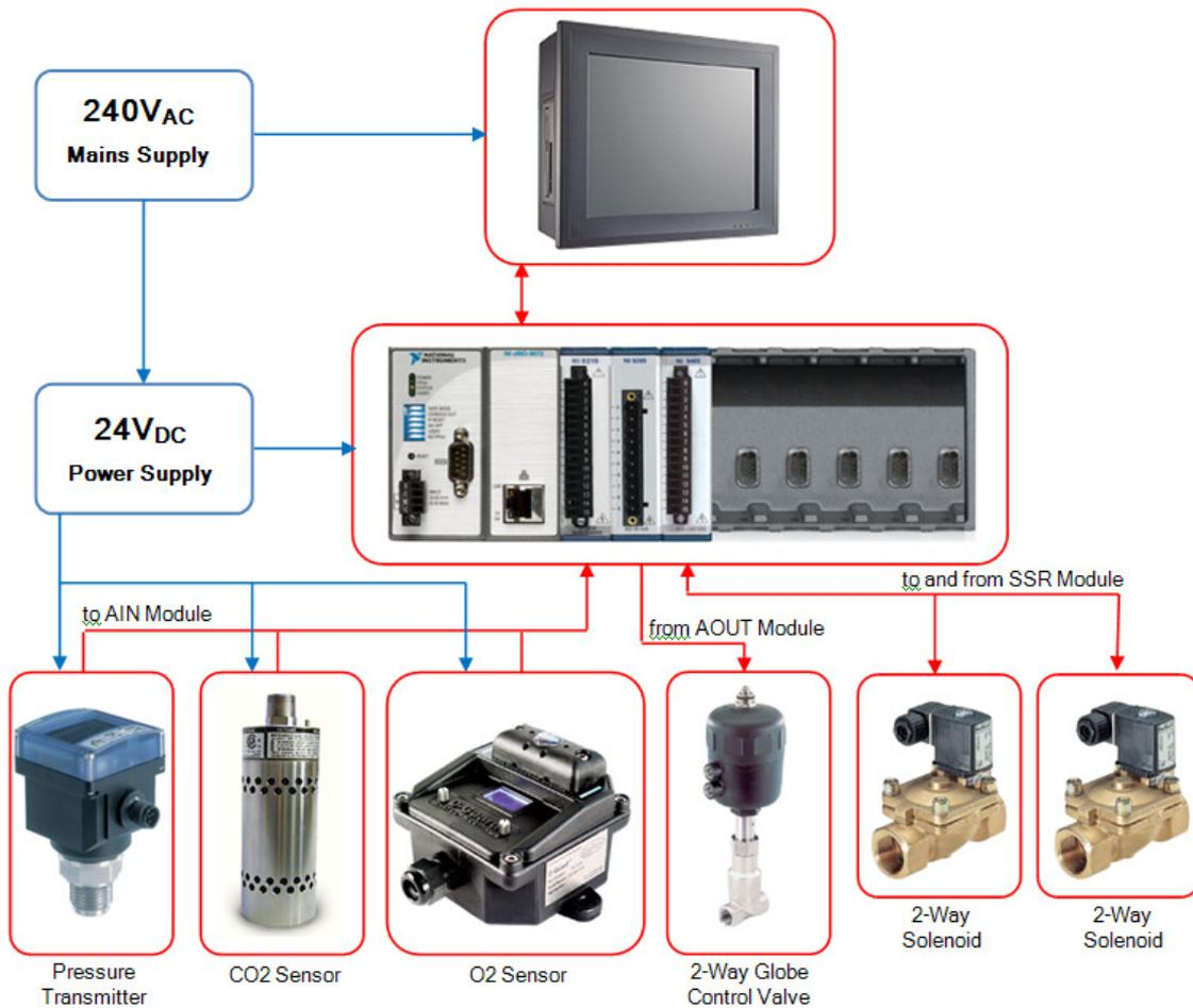
Figure 5 – Control System Architecture
